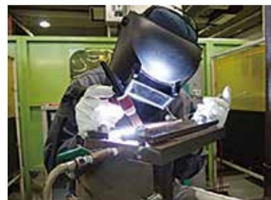
[治具を用いた下向き突合せ溶接]
