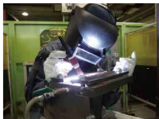
[治具を用いた下向き突合せ溶接]
